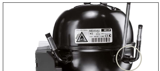
DELTA compressor with copper (suction, process) and copper-plated steel (discharge) connectors
