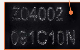
Fig.13 Needle print coding on compressor housing and country of origin on type label
